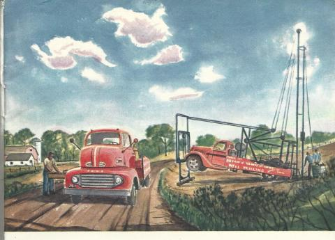
The Bryan Lewis drilling rig literally "picks itself up by its bootstraps." An F-6 equipment truck is on the left.
