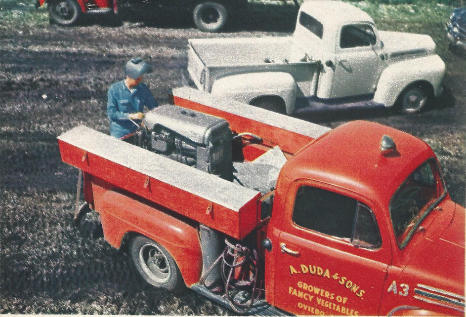
This F-2 service wagon is ready at all times to make emergency repairs in the field. It carries welding equipment and a complete tool kit.
