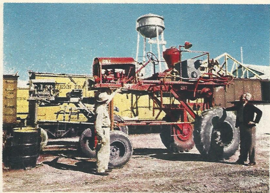
The machine at left is an F-5 on stilts used to pollenate corn. John Duda (in khakis) explains his duster to the Ford representative.
