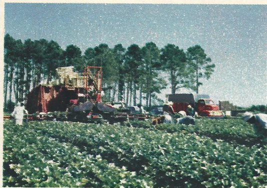
Rube Goldberg might have invented this weird harvester, left, which picks, washes, and crates crops of prime celery.
