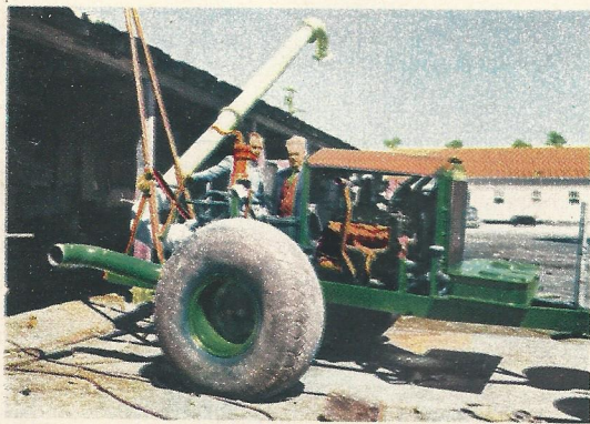
The Dudas built the portable irrigation pump at left in their machine shop. It is powered by a Ford V-8 industrial engine.
